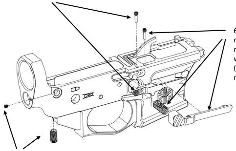
6. Install standard AR-15 magazine release spring and magazine release then secure with threaded pivot pin.
