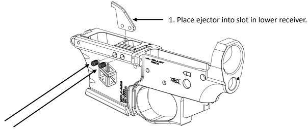
2. Using a 3/32" Allen drive, install extended-tip set screws. Ensure set screw tips seat into the holes in the ejector. <u>Torque screws to 15 in-lbs</u>. Use of blue Loctite is recommended.
