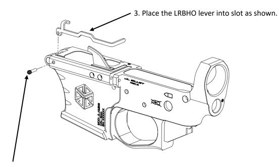
4. Using a 1/16" Allen drive, install threaded pivot pin into lower as shown to secure lever.
